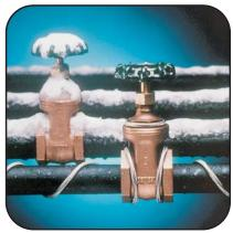
Constant Wattage Cable This style of heat trace cable is designed to put out a certain amount of wattage per linear foot at a particular voltage. It is always putting out the designed watts per foot, no matter what the surface or ambient temperature is.
